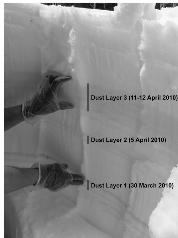
Fig. 2. Photograph showing dust layers deposited across the central Wasatch on 30 March, 5 April, and 11–12 April 2010.
