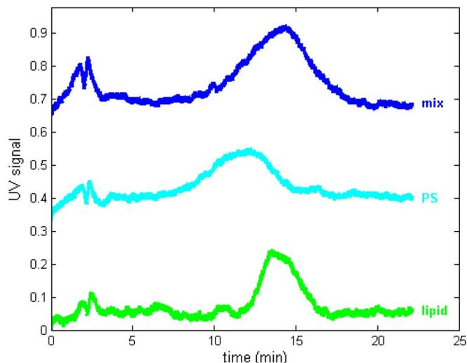
Fig. 4. UV fractograms of 100 nm lipid and polystyrene sulfonate (PS) coated magnetite nanoparticles (exp4). Voltage: 10 Vpp, 5 Hz, 70% duty cycle. Flow: 1 ml/min.
