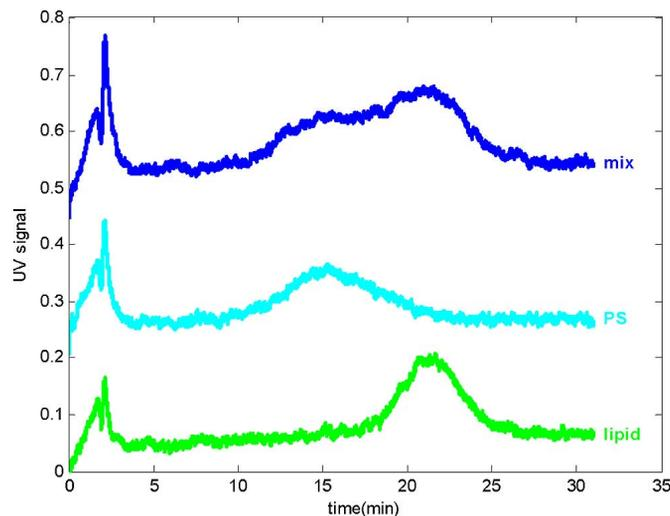
Fig. 5. UV fractograms of 50 nm lipid and polystyrene sulfonate (PS) coated magnetite nanoparticles (exp5). Voltage: 6 Vpp, 10 Hz, 75% duty cycle. Flow: 1 ml/min.
