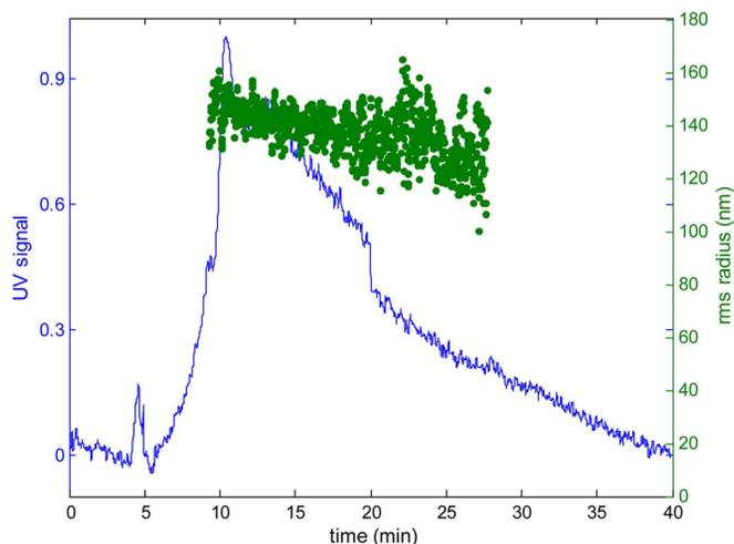
Fig. 3. UV absorption fractogram and rms radius data of the MACS nanoparticles (exp3). Voltage: 10 Vpp, 10 Hz, 60% duty cycle. Flow: 0.5 ml/min.
