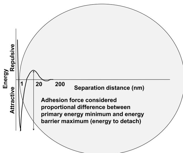
**Figure 2.** Schematic of colloid-surface interaction force profile superimposed on colloid of  $\sim 800$  nm diameter associated with the surface via the primary energy minimum.
