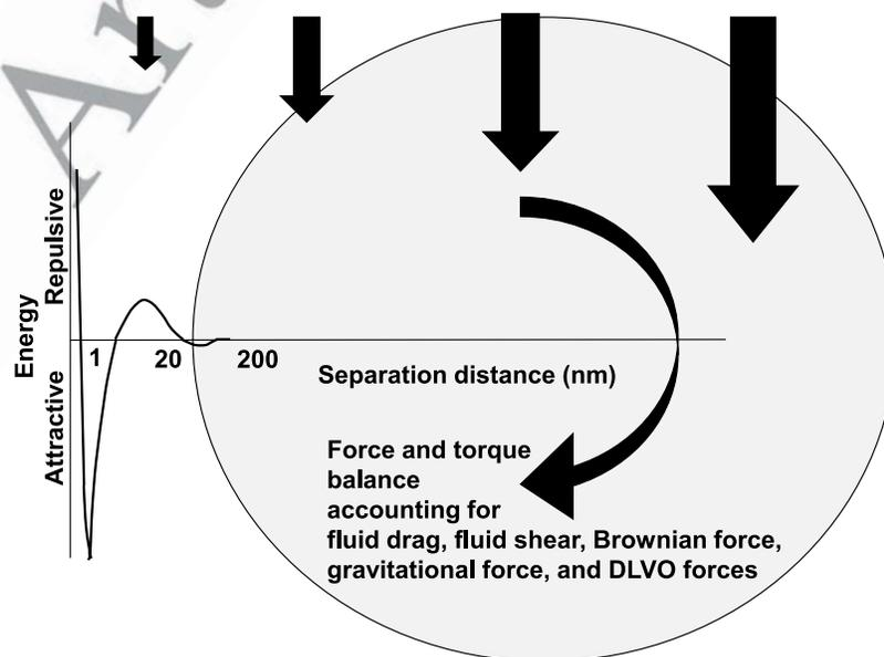
**Figure 3.** Schematic of colloid-surface interaction force profile superimposed on colloid of  $\sim 800$  nm diameter associated with the surface via the secondary energy minimum. Arrows depict fluid drag force and associated torque.
