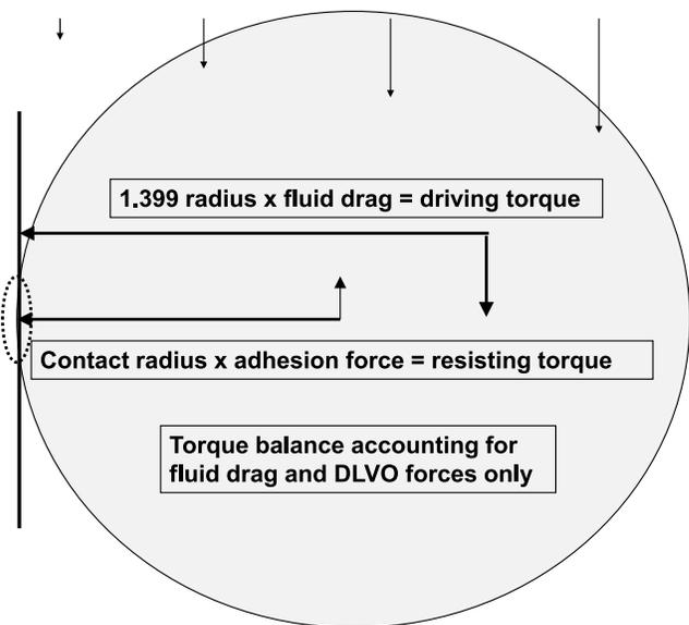
**Figure 1.** Schematic of colloid attached to surface with corresponding driving torque (driving detachment) originating from fluid drag (depicted by arrows at top) and resisting torque (resisting detachment) originating from adhesion.
