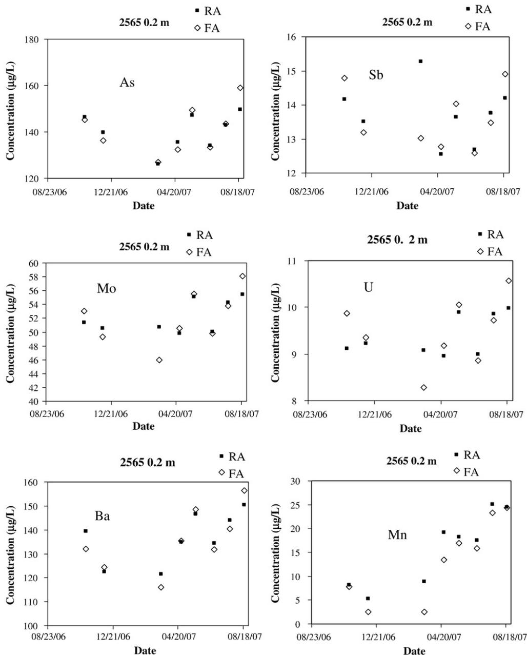
Fig. 4—Selected trace metals trajectories measured via CC-ICP-MS for shallow brines represented by site 2565 at 0.2 m.
