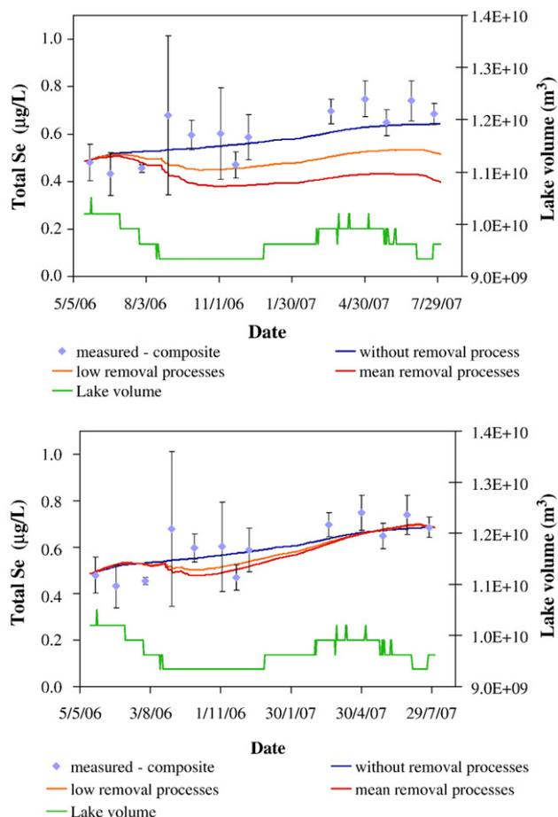
**Fig. 3** – Mass balance integration of Se concentration in the Great Salt Lake. **Top:** using estimated loads and removal processes. **Bottom:** adding estimated unmeasured loads to reach the July/07 target Se concentration. [Se] measured stands for composite data from 4 sites and all shallow depths.
